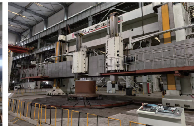
Ck52125 数控双柱立式车床 12.5 meters Double Column Vertical lathe
