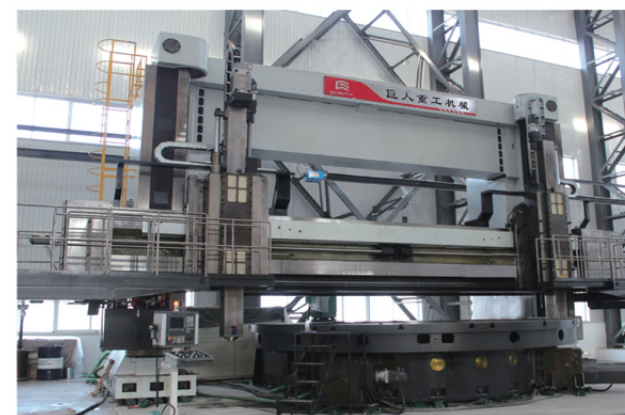
CXK5280 数控双柱立式车铣复合机床 8 meters vertical turning and milling machine
