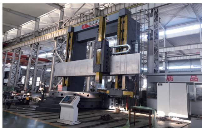
CK5250 数控双柱立式车床 5 meters vertical lathe with side tool post
