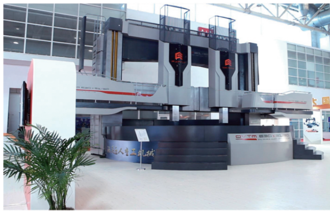
CXK5263 数控双柱立式车铣复合 6.3 meters vertical turning and milling machine To Russia customer
