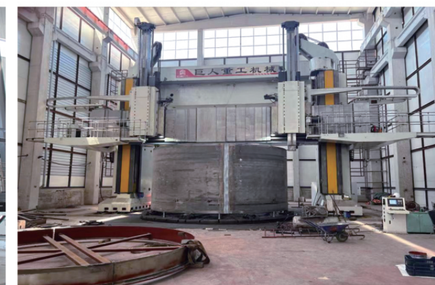
CXK52100 立式车铣复合加工中心 10 meters vertical turning and milling machine
