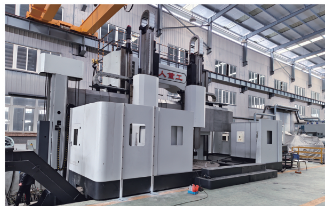
CXK5240 数控双柱立式车铣复合 4 meters vertical turning and milling machine
